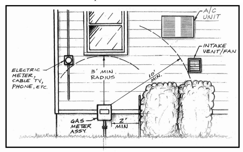
The measurements shown above are intended as a guide and represent minimum clearances. NPU reserves the right to approve the final meter location.
