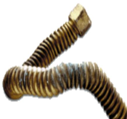
**Gas connectors should be inspected regularly and replaced as needed. Certain types of flexible connectors manufactured between 1970 and 1980 may fail over time and need to be replaced.**
